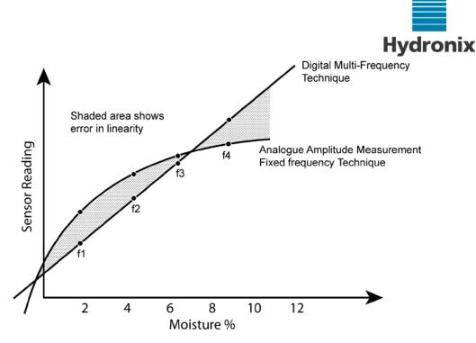
Figure 3: The effects of a non-linear measurement technique
