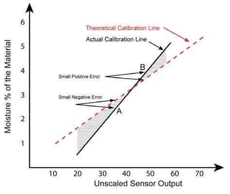
Figure 4: The effects of assuming a calibration slope
