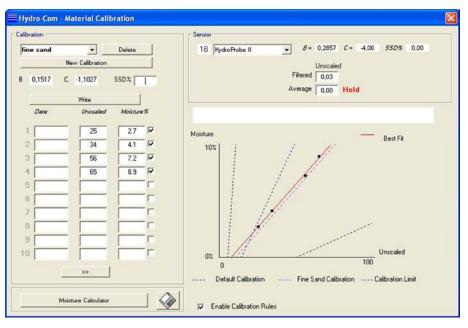
Figure 5: A multi-point calibration technique is recommended
