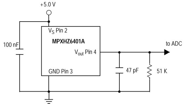
Figure 3. Typical Application Circuit (Output Source Current Operation)
