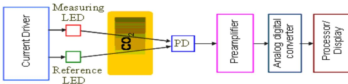
There are strong absorption bands of many chemical agents at mid-infrared spectral range that allow their detection with sensor devices based on LED-PD optopairs. Some of these chemical agents and their absorption bands are presented here:
