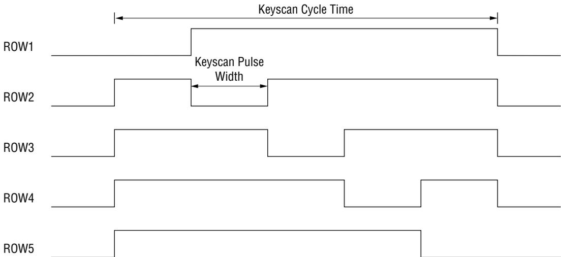
**Output Timing (Duplex Operation)** \*1bit time=4/f<sub>OSC</sub>
