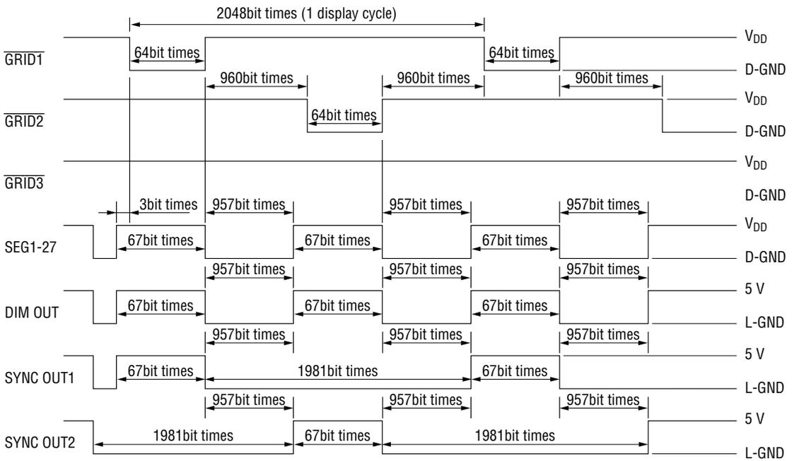
**Output Timing (Triplex Operation)** \*1bit time=4/f<sub>OSC</sub>
