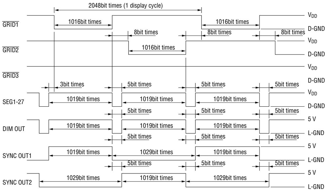
**Output Timing (Triplex Operation)** \*1bit time=4/f<sub>OSC</sub>
