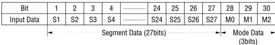
[Bit correspondence between segment output and segment data]
