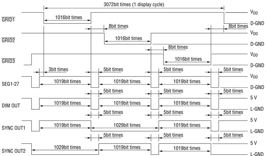
**Output Timing (Duplex Operation)** \*1bit time=4/f<sub>OSC</sub>
