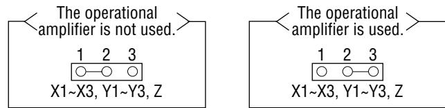
With the operational amplifier not used, I+, I-, Q+, Q- and ENV output signals of MSM7583 are given out directly at the BNC terminals on the board. With the operational amplifier used, the addition of I+ and I- is output at I+ of the BNC terminal, the addition of Q+ and Q- at Q+, and buffered ENV output at ENV of the BNC terminal.
