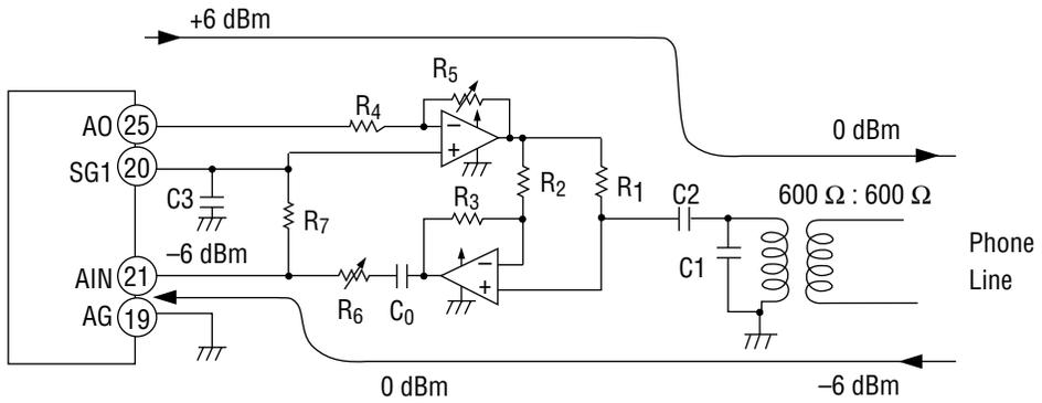
Figure 9 MSM6926RS/MSM6946RS Application
