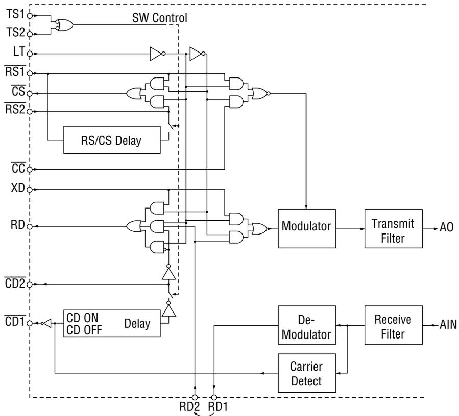
Figure 12 Equivalent Logic Interface of the Integrated Modem
