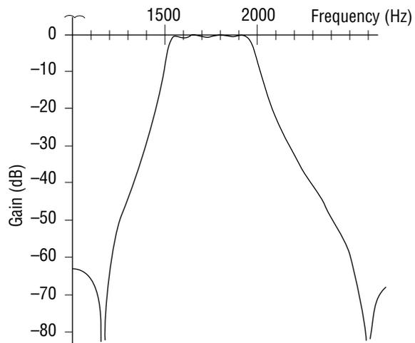
Figure 3 MSM6926 High Band Filter
