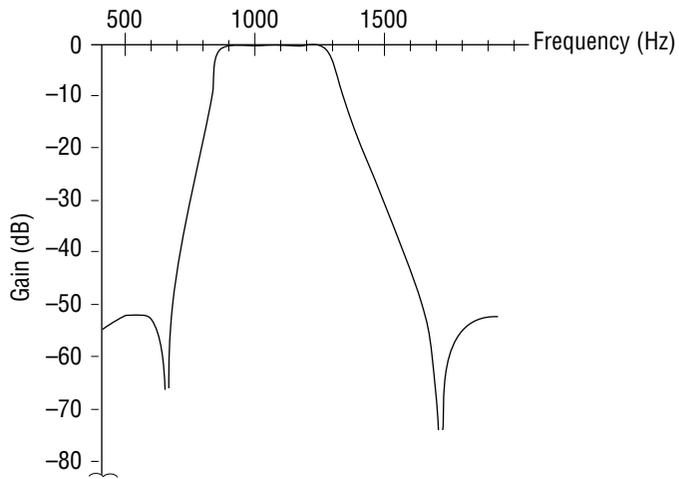
Figure 2 MSM6926 Low Band Filter
