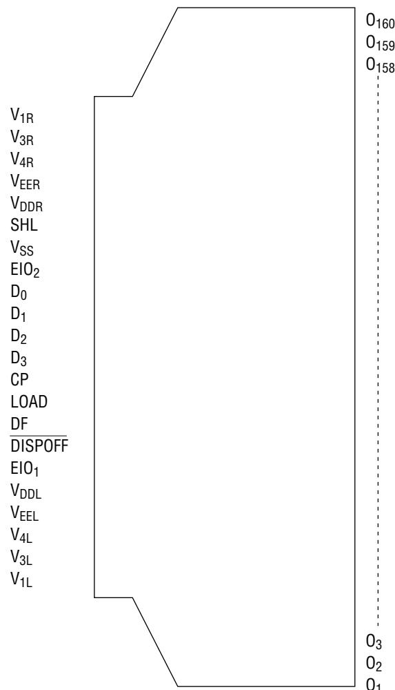
Note: The drawing shown does not specify the exact outline of the TCP; it only specifies the pin layout.
