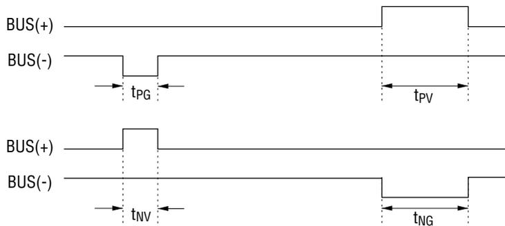
Reset Input Pulse Width
