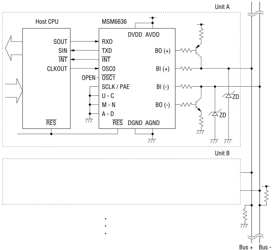
The above connection example is when "UART, MPC and parity no mode" was used as the "host CPU interface, and when CLKOUT output of the host CPU" was used as the clock for MSM6636.
