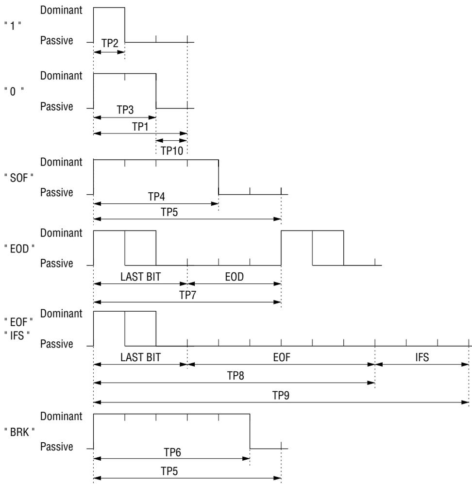
CPU Serial Interface Timing
