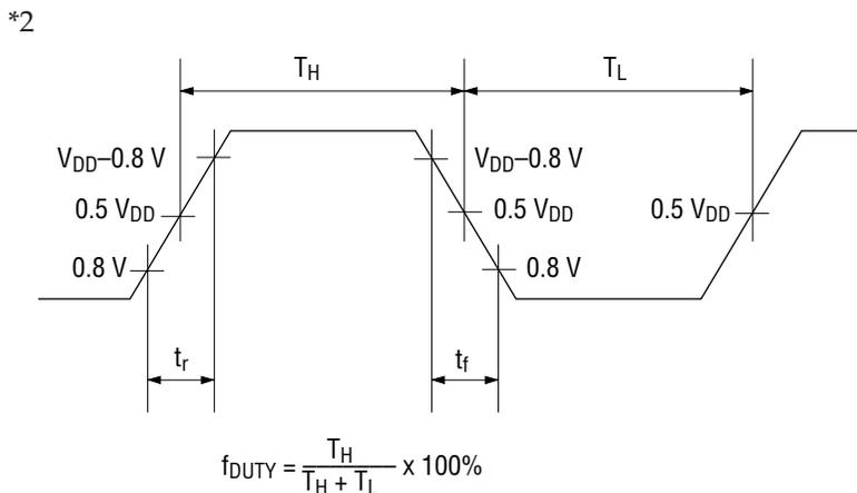
**TIMING DIAGRAM****Interface with 80 Series CPU** $(V_{DD} = 4.5 \text{ to } 5.5\text{V}, T_a = -20 \text{ to } +75^\circ\text{C})$
