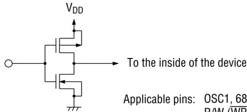
Applicable pins: OSC1, 68 series/80 series,  $\overline{CS}$
