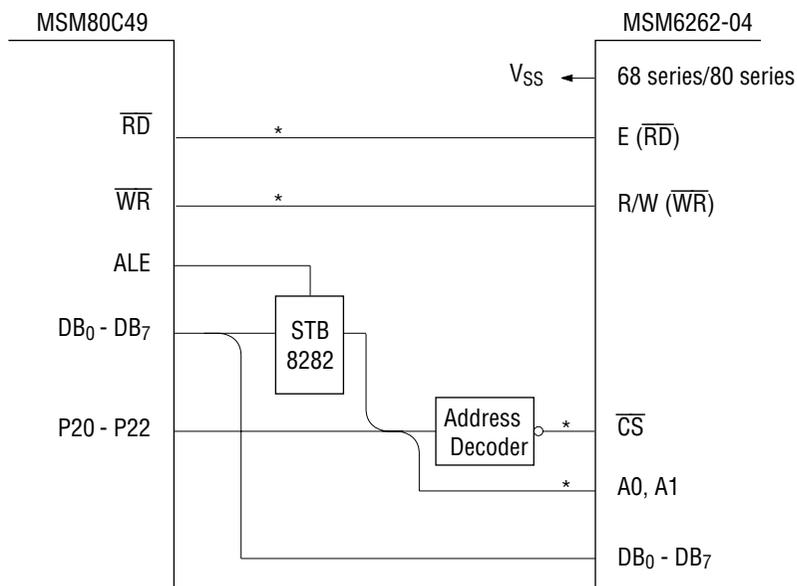
\* A pull-up resistor of about 50 kΩ is required when the output of CPU becomes high impedance.
