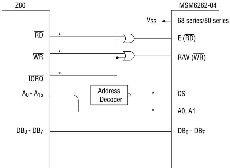
\* A pull-up resistor of about 50 k $\Omega$  is required when the output of CPU becomes high impedance.
