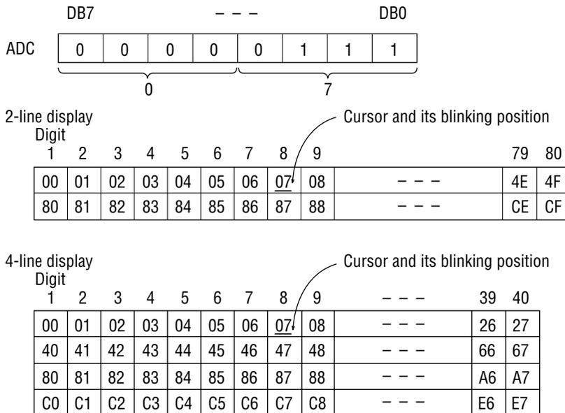
Note: Cursor display and blinking can be performed even when the CG RAM address is set in the ADC. So, it is necessary to disable the cursor display and blinking when the CG RAM address is set in the ADC.
