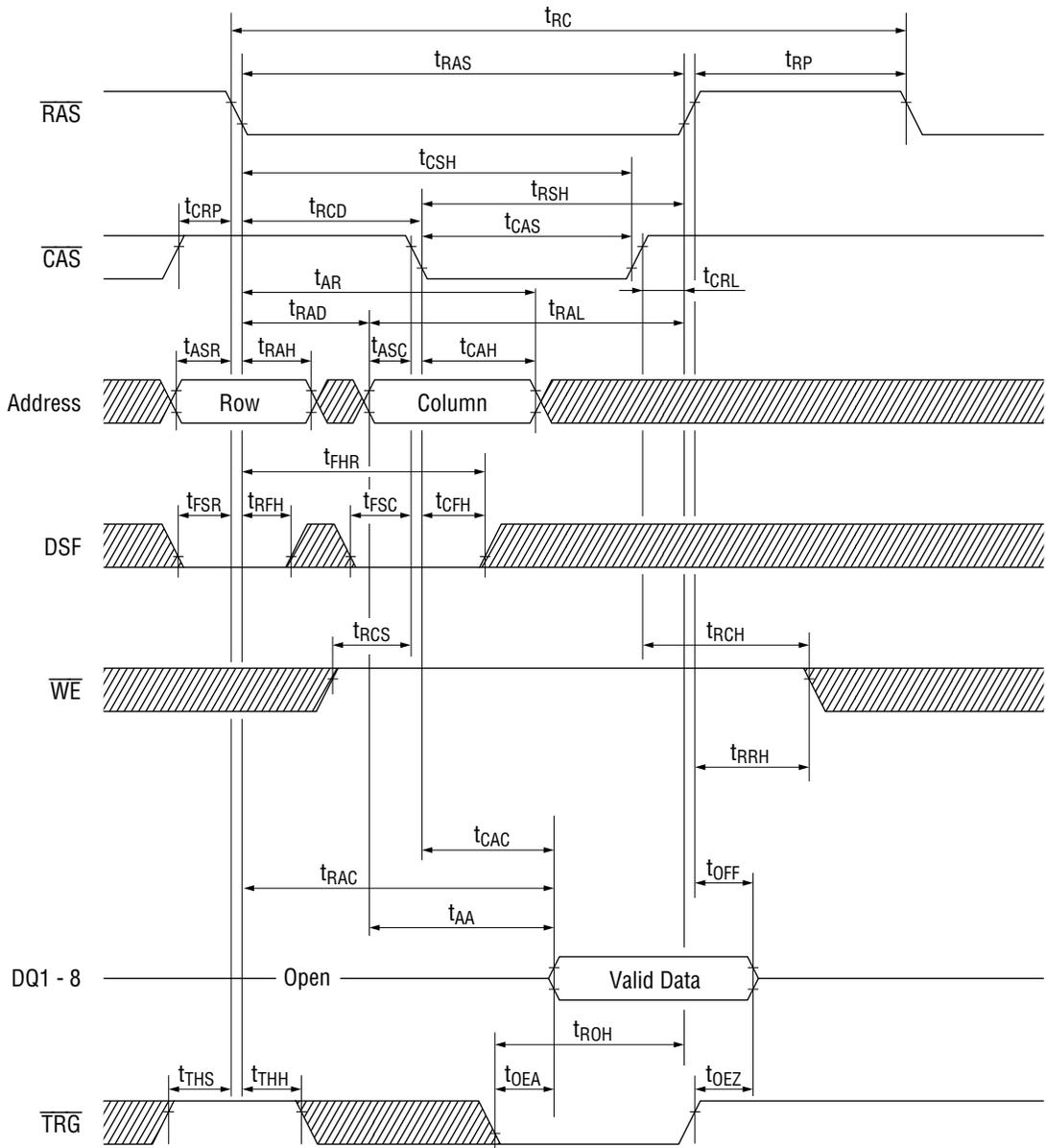
Read Cycle (Outputs Controlled by  $\overline{\text{CAS}}$ )
