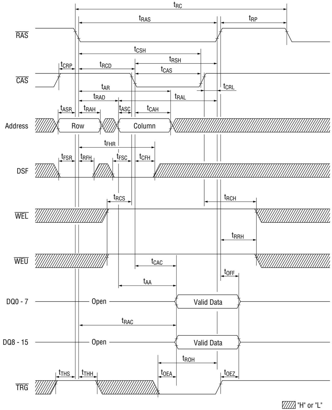
Read Cycle (Outputs Controlled by  $\overline{\text{CAS}}$ )
