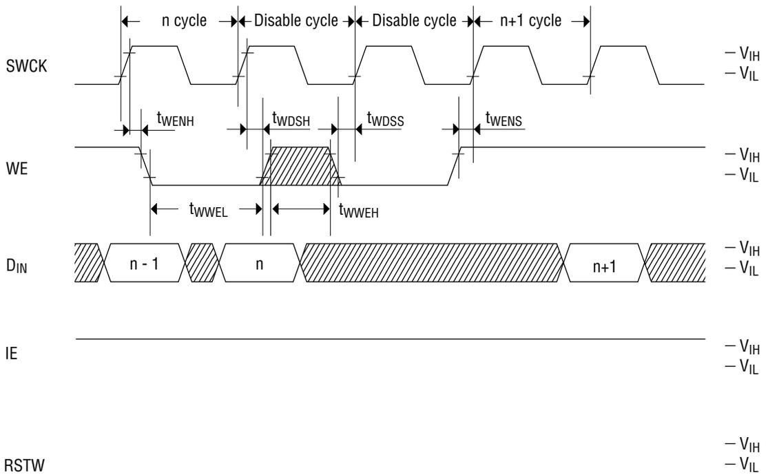
**Write Cycle Timing (Input Enable)**
