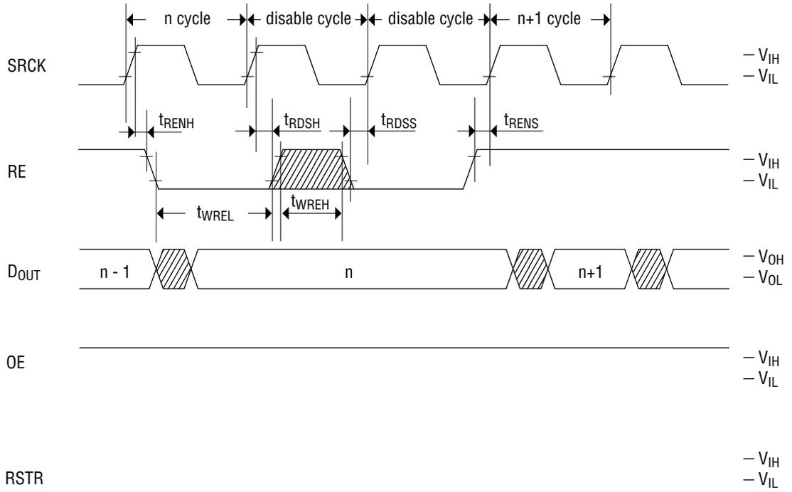
**Read Cycle Timing (Output Enable)**
