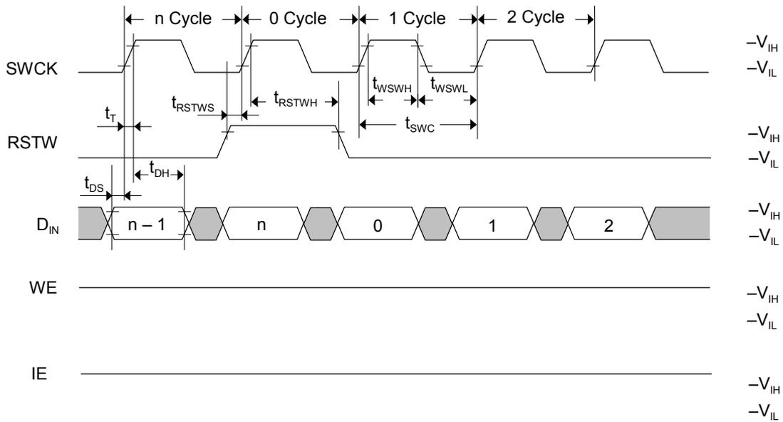
**Write Cycle Timing (Write Enable)**
