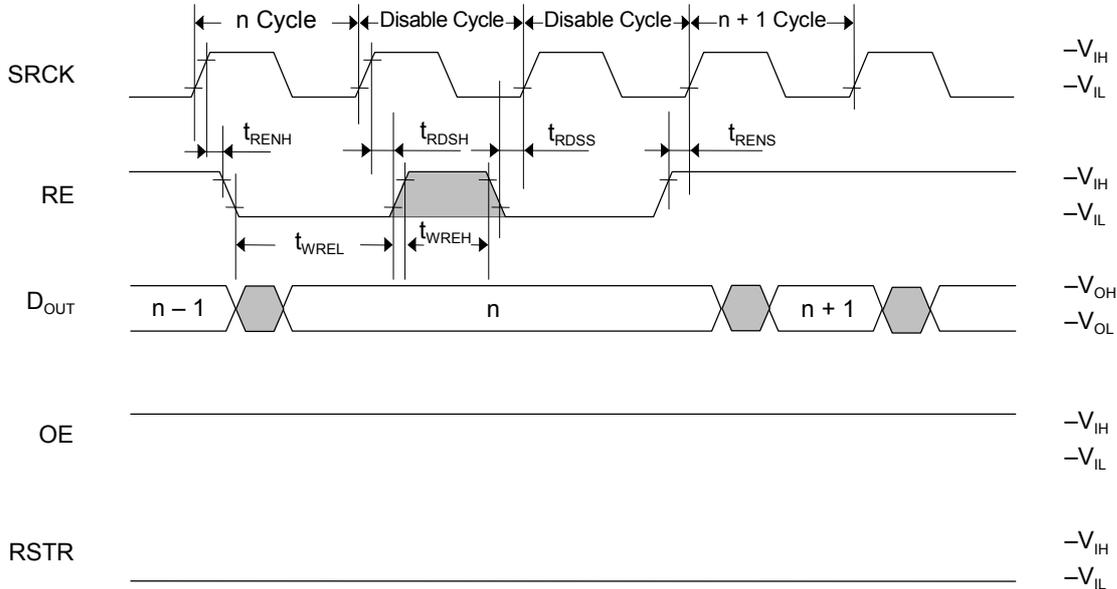
Read Cycle Timing (Output Enable)
