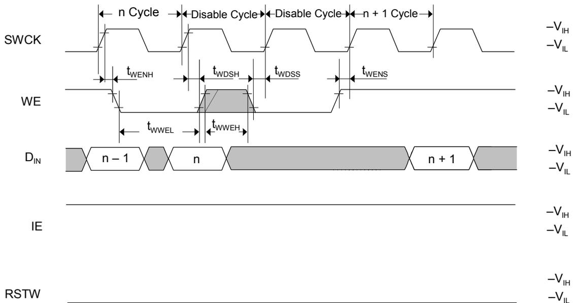
**Write Cycle Timing (Input Enable)**
