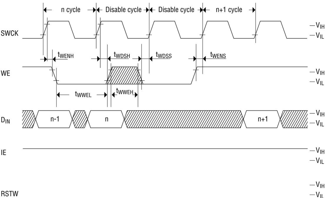
**Write Cycle Timing (Input Enable)**
