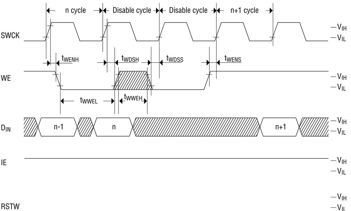
**Write Cycle Timing (Input Enable)**
