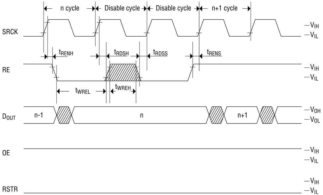
**Read Cycle Timing (Output Enable)**
