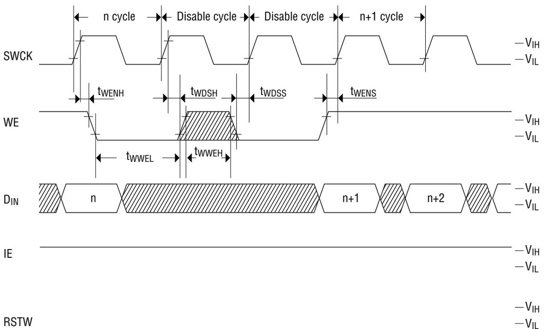
**Write Cycle Timing (Input Enable)**
