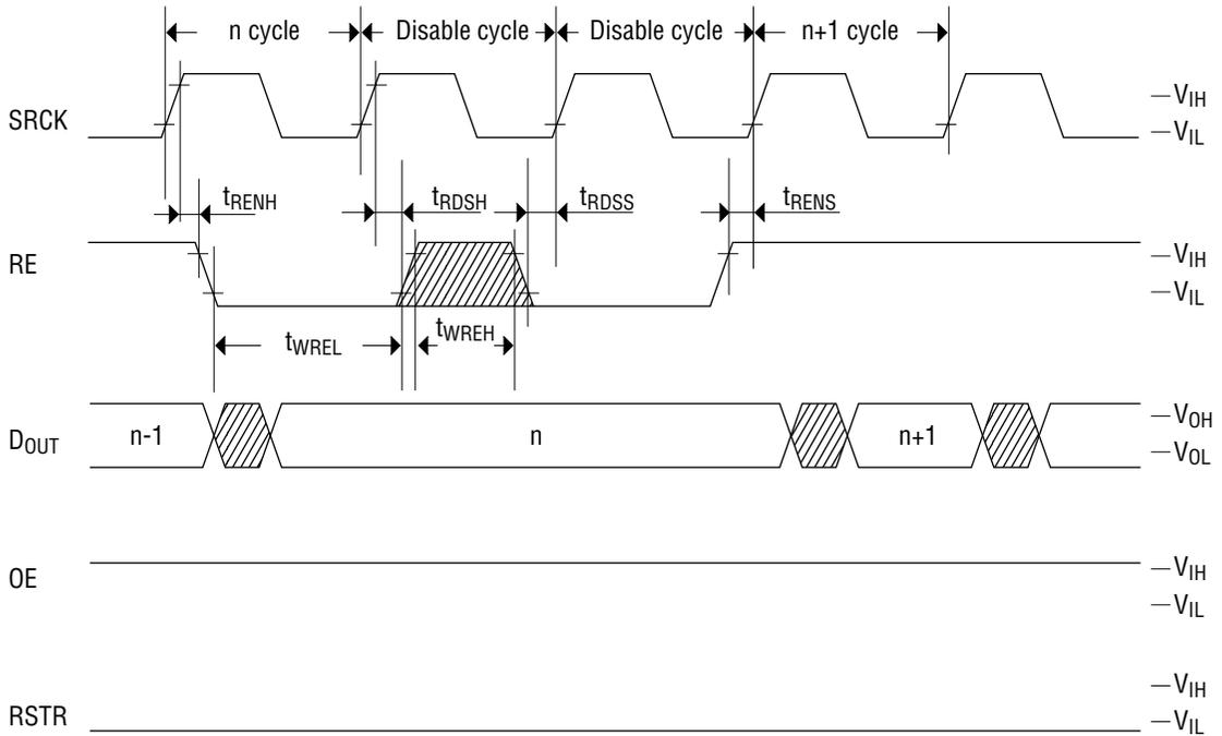
**Read Cycle Timing (Output Enable)**
