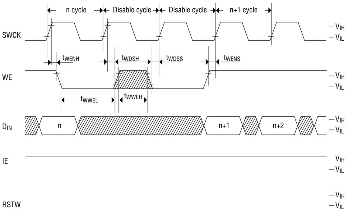
**Write Cycle Timing (Input Enable)**
