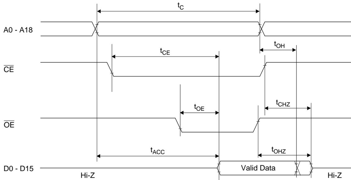
8-Bit Read Mode ( $\overline{\text{BYTE}} = V_{IL}$ )
