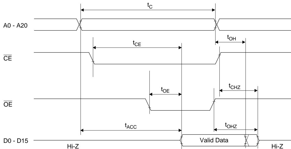
8-Bit Read Mode ( $\overline{\text{BYTE}}=V_{IL}$ )
