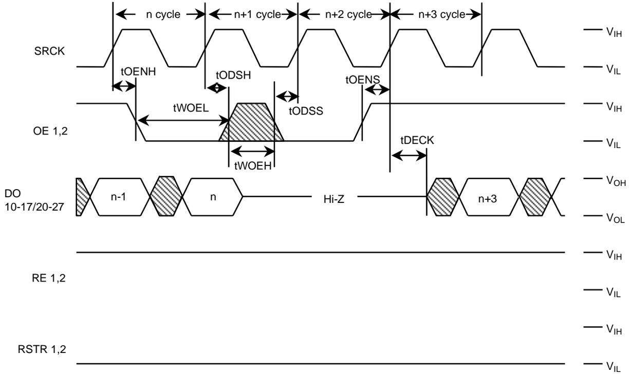
**Read Cycle Timing (Read Reset) : MODE1=Vcc/Vss , MODE2=Vcc**
