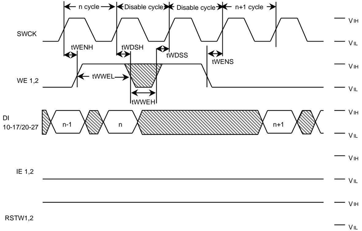
**Write Cycle Timing (Input Enable) : MODE1=Vcc , MODE2=Vcc**
