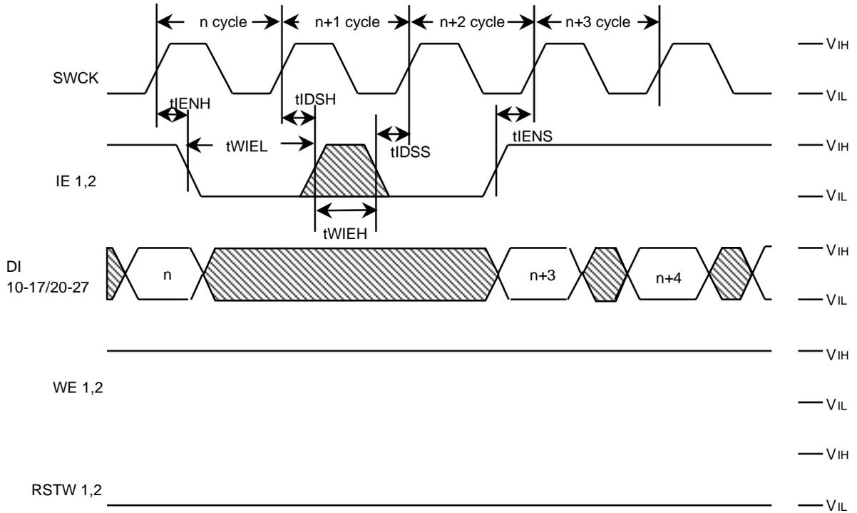
**Write Cycle Timing (Write Reset) : MODE1=Vss , MODE2=Vcc**
