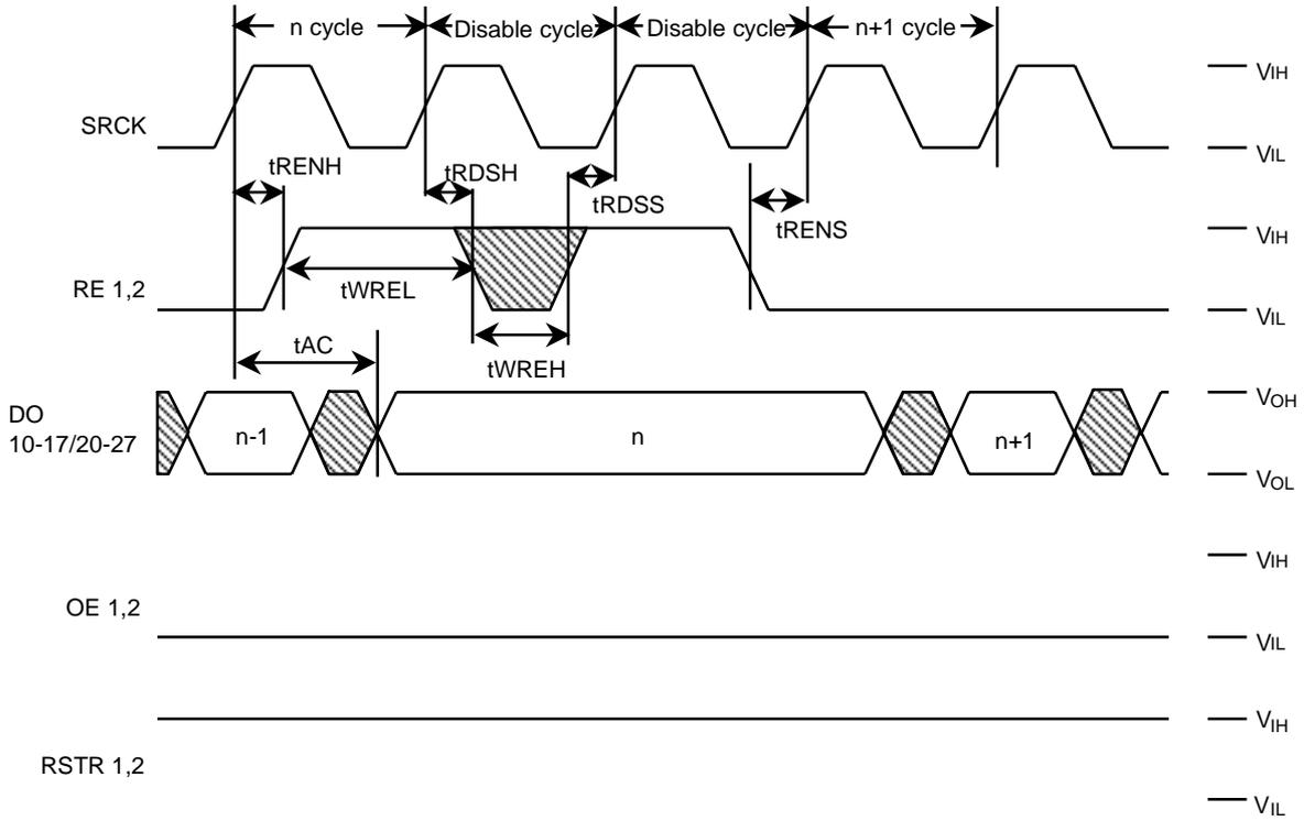
**Read Cycle Timing (Output Enable) : MODE1=Vcc/Vss , MODE2=Vcc**
