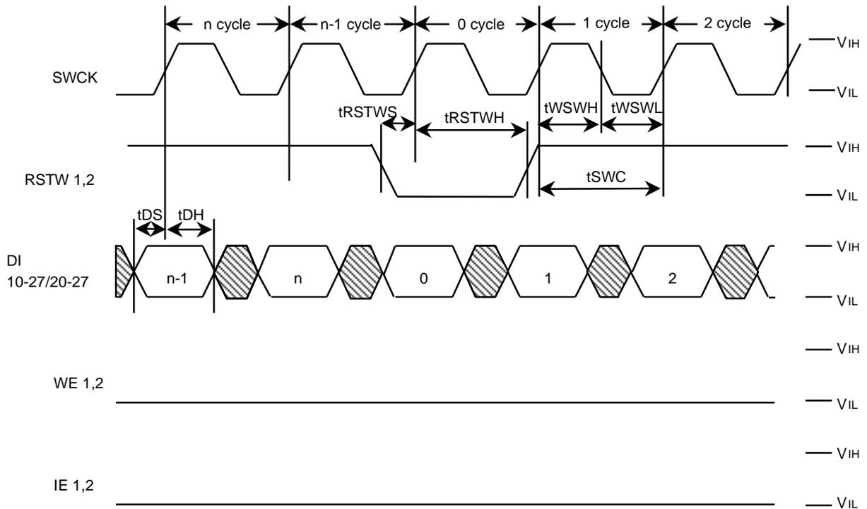
**Write Cycle Timing (Write Enable) : MODE1=Vss , MODE2=Vcc**
