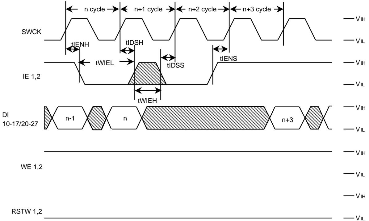
**Write Cycle Timing (Write Reset) : MODE1=Vcc , MODE2=Vcc**
