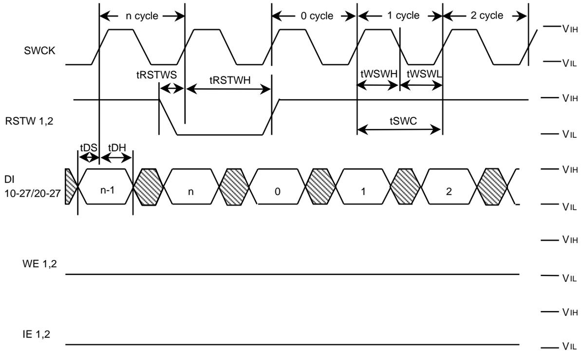
**Write Cycle Timing (Write Enable) : MODE1=Vcc , MODE2=Vcc**
