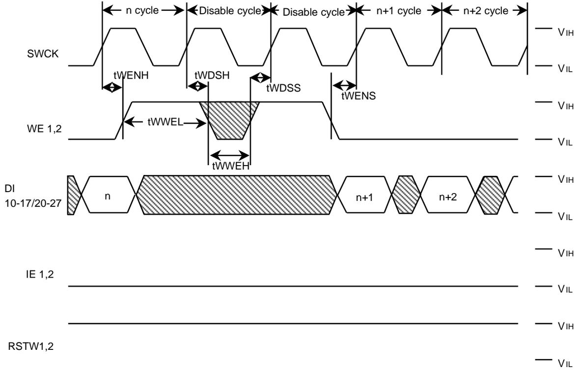
**Write Cycle Timing (Input Enable) : MODE1=Vss , MODE2=Vcc**
