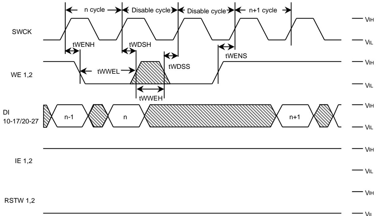
**Write Cycle Timing (Input Enable) : MODE1=Vcc , MODE2=Vss**
