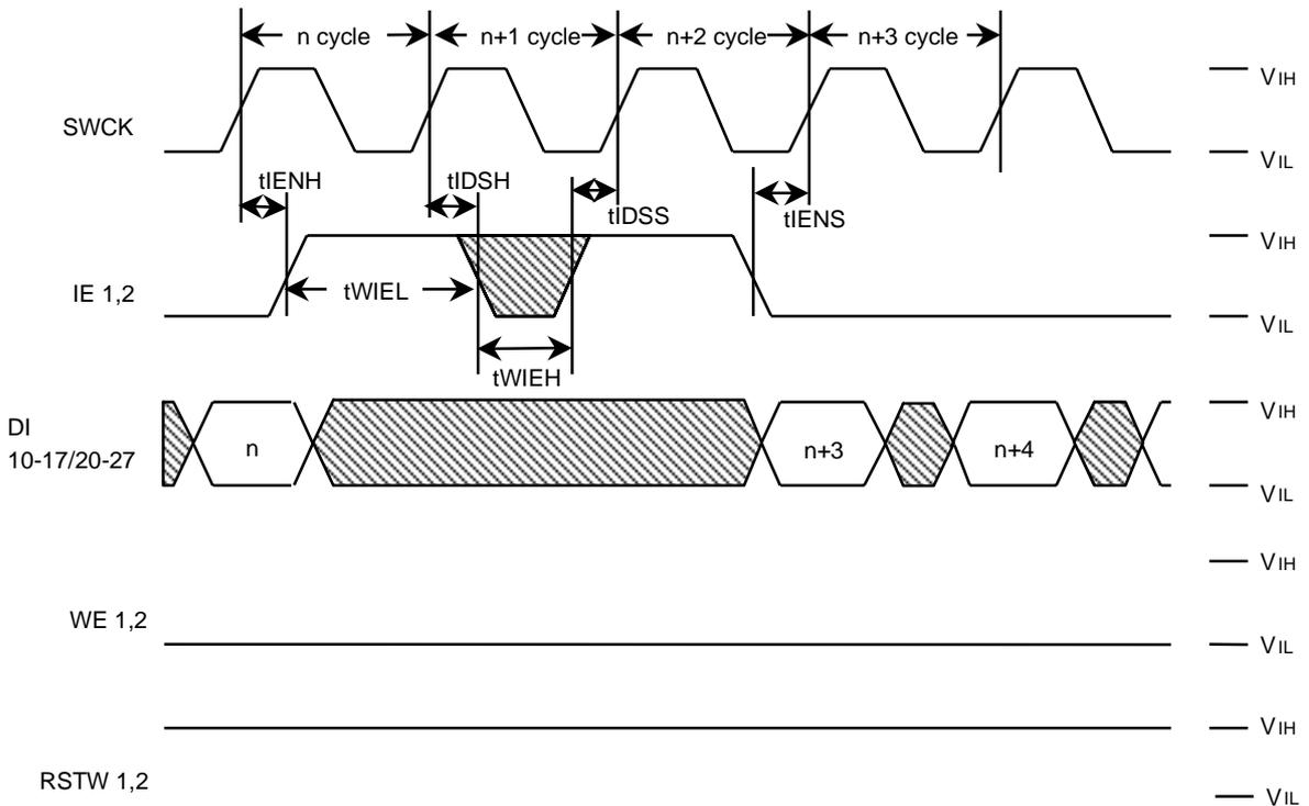
**Read Cycle Timing (Output Enable) : MODE1=Vcc/Vss , MODE2=Vss**
