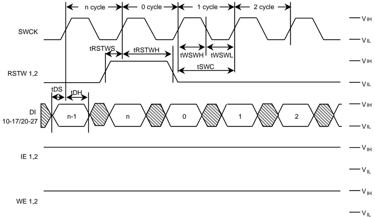
**Write Cycle Timing (Write Enable) : MODE1=Vcc , MODE2=Vss**
