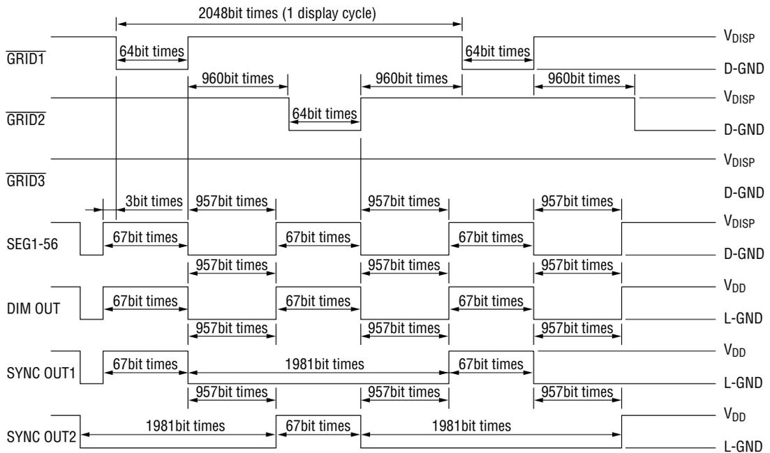
● **Output Timing (Triplex Operation)** \*1bit time=4/f<sub>OSC</sub>
