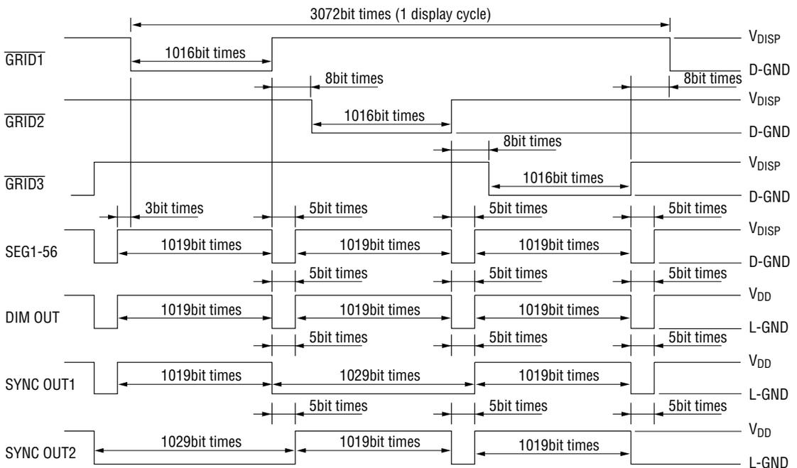
● **Output Timing (Duplex Operation)** \*1bit time=4/f<sub>OSC</sub>
