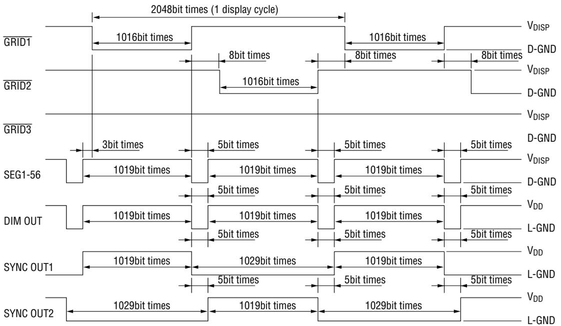
● **Output Timing (Triplex Operation)** \*1bit time=4/f<sub>OSC</sub>
