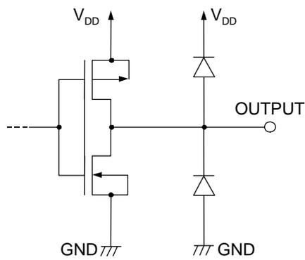
**Schematic Diagram of Driver Output Circuit**
