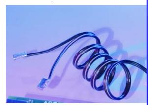
The Electrostatic Cable assembly, usually a component part of the 6500 Sonar Ranging Module, contains clips to connect between the Series 600 (or the Series 7000) Electrostatic Transducer and the 6500 Sonar Ranging Module's drive electronics. The Black (with color stripe) lead is connected to GND, and connects to the minus (-) transducer connection.
