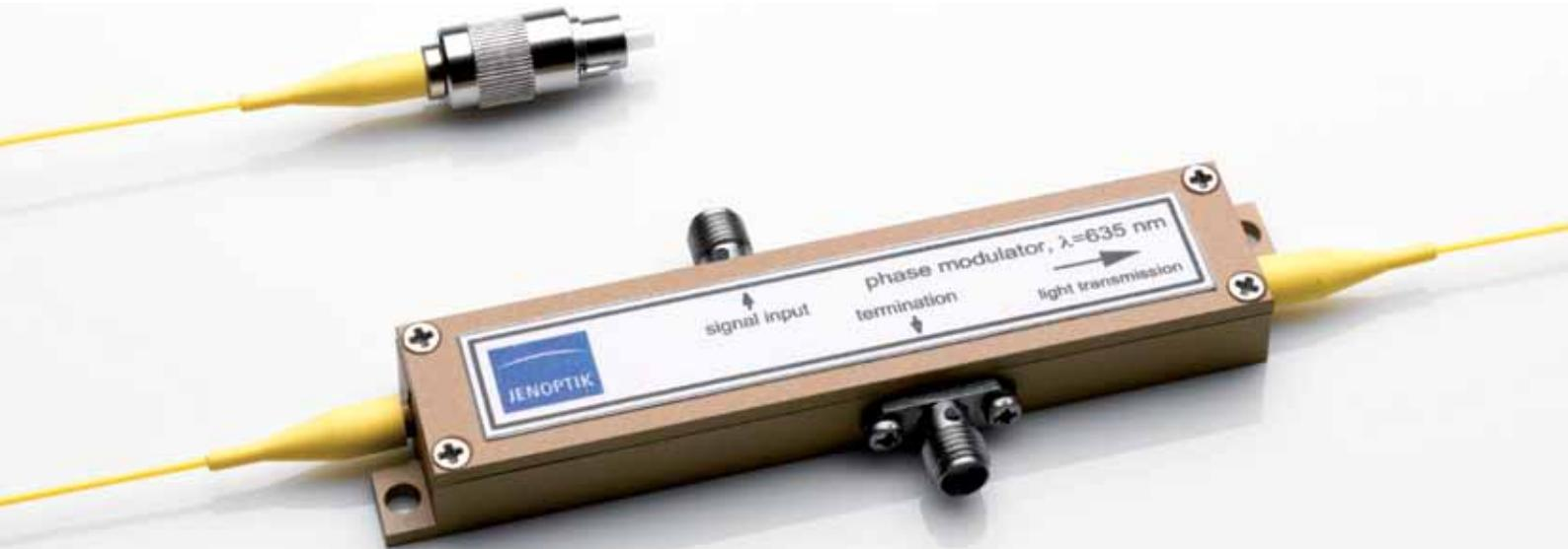
The Integrated Optical Phase Modulator is a compact fiber-coupled electro-optical modulator that works based on MgO:LiNbO<sub>3</sub> and LiNbO<sub>3</sub> crystals. Providing fast electro-optical response, it allows phase modulation with frequencies as high as the Gigahertz range. Available modulators can handle wavelengths in the visible and the infrared spectral range.
