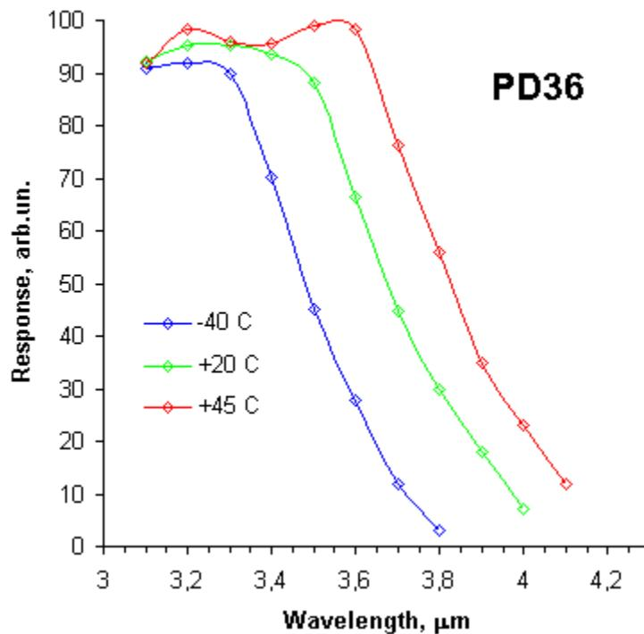
Long-wavelength edge of the spectra, measured at different temperatures and temperature dependence of the Impedance for PD36-02 is presented here. Temperature dependences of the other models have the same shape.
