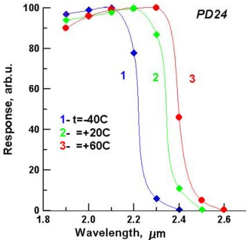
Long-wavelength edge of the spectra, measured at different temperatures and temperature dependence of the dark current for PD24-02 is presented here. Temperature dependences of the other models have the same shape.
