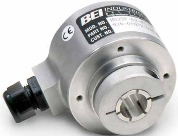
The HS25 combines the rugged, heavy-duty features usually associated with shafted encoders into a hollow-shaft style. Its design includes dual bearings and shaft seals for NEMA 4, 13 and IP65 environmental ratings, a rugged metal housing, and a cable gland.
