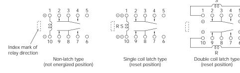
S: Coil polarity of set (operate) R: Coil polarity of reset (release)
