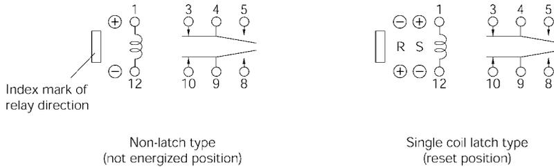
S : Coil polarity of set (operate)
