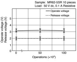
Ambient temperature: Room temperature Driving: 5 V dc, 2 Hz, 50% duty
