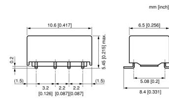
Tolerance of lead pitch is : ±0.15 mm [0.006inch] Another tolerance is ±0.3 mm [0.012 inch] ( ) is reference value.
