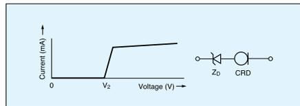
**The compensation of current reduction due to self heating**
