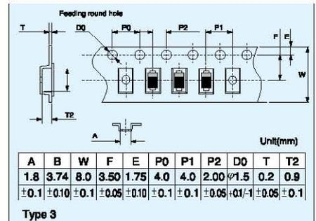
\*In principal elements are set with cathode side on the round hole side.
