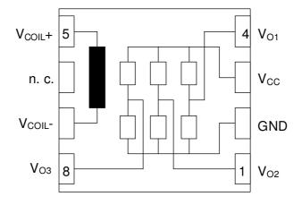
Figure 1: internal and external connections (TDFN, Chip)
