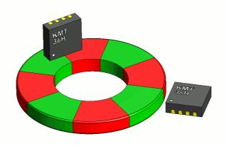
As an unique feature, the KMT36H is able to measure full 360° by utilizing an additional magnetic field which is generated by a planar coil which is located on the chip. The 180°/360° determination is done by a simple sign distinction and may be proceeded periodically or only once at power up.
