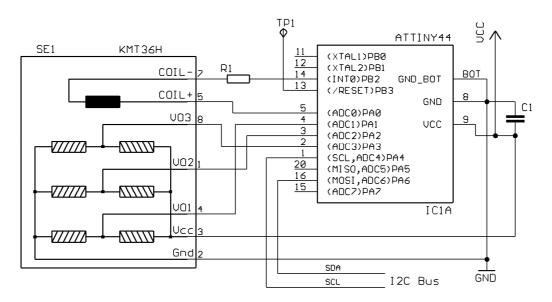
Figure 5: One exemplary hardware configuration using an Atmel ATtiny μC
