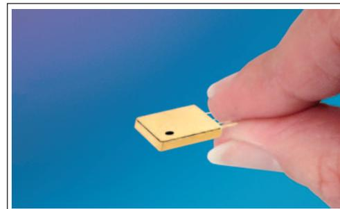
The LLE-1-500 series transducers are an excellent solution for Wind Tunnel, Flight Test, Nozzle (vectoring, etc.), and Fuselage pressure measurement applications. Their light weight and flat packaging makes them especially suitable for direct adherence to test parts where other means of pressure sensor installation are undesirable or not possible. These transducers incorporate the latest Kulite patented and patent pending technologies in pressure sensor development.
