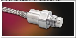
back of the metal flush diaphragm. Incorporation of Kulite proprietary high temperature 500°F (437°F continuous) electronics within the main body allows for operation from an unregulated power supply of 10 to 36 VDC.
