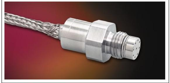
non-compressible silicone oil. This sensing sub-assembly is protected from mechanical damage by a protective screen, which has been shown to have minimal influence of the frequency response of the sensor. Incorporation of Kulite proprietary high temperature 500°F (437°F continuous) electronics within the main body allows for operation from an unregulated power supply of 10 to 36 VDC.
