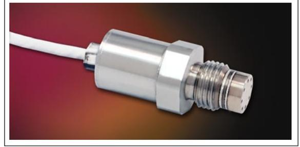
The ETL-UHT-375M is one of the newest generation of Kulite standard, smallest ultra high temperature miniature amplified transducer currently available. The device incorporates Silicon on Insulator (SOI) Sensor and Electronics, thus enabling operation up to 450°F (232°C). The ETL Series uses Kulite's Patented Leadless Technology. This sensing sub-assembly is protected from mechanical damage by a protective screen, which has been
