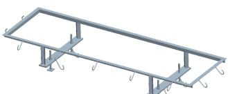
Fig. 4: Mounting frame – External dimensions (including anchors) (LxWxH) = 3240x1150x475 mm, weight = 80 kg
