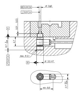
Fig. 3: Mounting in blind hole with measuring pin and hardened thrust washer  $\emptyset$ 3,5 mm Type 9406
