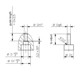
Fig. 4: Hole and dimensions of the measuring pin
