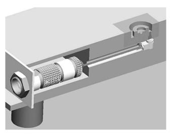
Fig. 8: Installation with sensor, measurement pin, cable, connector and mounting plate
