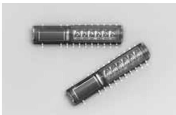
[Figure 5-7] Light emitting/receiving module P8212 for VICS
