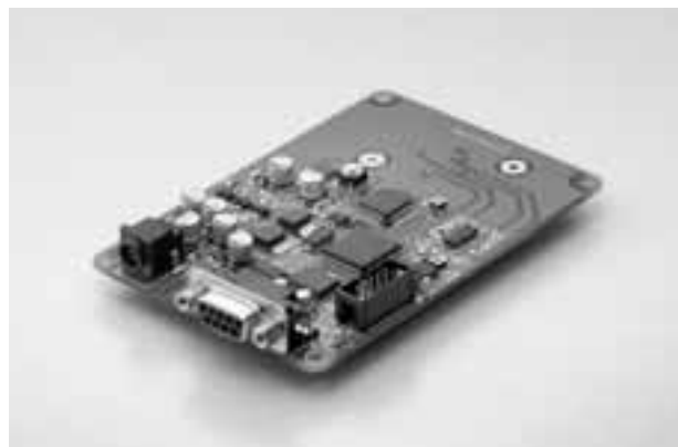
[Figure 4-23] Two-dimensional PSD signal processing circuit C9069
