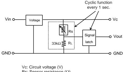
Rs: Sensor resistance ( $\Omega$ ) RL: Load resistance ( $\Omega$ ) The sensor's output signal (Vout) and the circuit voltage (Vc) can be monitored through the Vout-GND and Vc-GND terminals respectively whenever a power source of 10VDC is applied. An input impedance of more than 1M $\Omega$  should be connected to the Vout-GND terminals in order to make precise data acquisition. Please refer to **Product Information for TGS2442** for a full description of the sensor's heating cycle.
