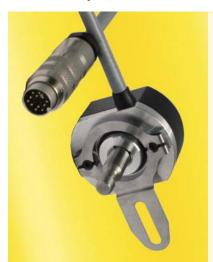
Designed as a drop in replacement for the Siemens 1XP8001 encoder, the DR686 is ready for delivery. The unique threaded shaft made this encoder hard to find, but now it is a standard order. Configurations can be ordered with either 1024 or 2048 CPR, with a 12 pin connector at the end of 18" of cable. Save time and money looking for a replacement encoder; The DR686 is the perfect solution!
