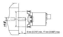
STEP 1 Slide the encoder over the motor shaft.
