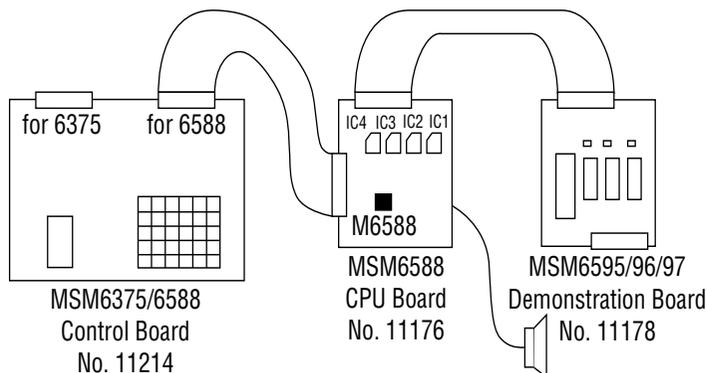
Note: When the serial register is not mounted to IC1 on the MSM6588 CPU board (No. 11176), the circuit does not operate normally. If serial register is mounted to IC2-IC4, the normal operation is not possible either.
