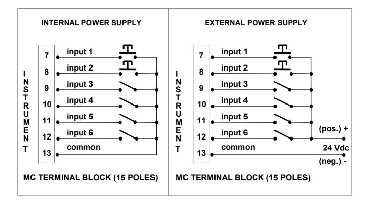
If the inputs have an external power supply, we recommend supplying them with a stabilized voltage, because a rectified voltage (pulsing) could cause constant input activation – de-activation.
