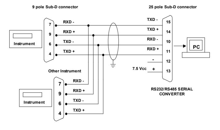
It should be born in mind that the last device connected must be terminated with a suitable resistance value. Make sure that this instrument is connected in the last place in the chain.
