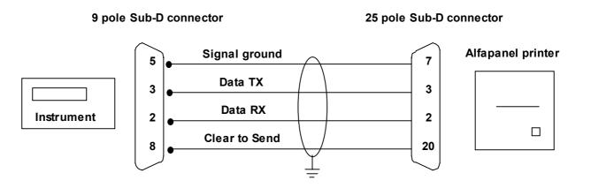
In the case of a printer equipped with a 9-pole connector instead of 25 the connections will be "pin to pin" (5  $\leftrightarrow$  5, 3  $\leftrightarrow$  3, 2  $\leftrightarrow$ 2, 8  $\leftrightarrow$  8).
