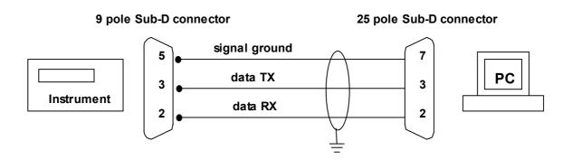
The diagram below illustrates connection of the instrument to a 9 pole PC connector:
