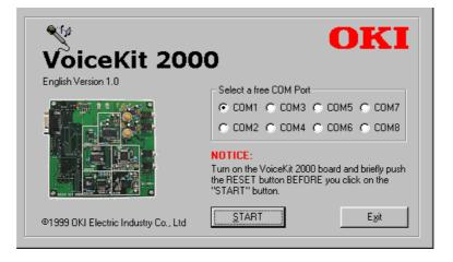
By default, COM1 is selected. Any valid selection you make will be stored in an initialisation file and be available at next start up. Before going further, please make sure that the serial cable is properly connected to both VK2000 and the host. Then engage power to VK2000 and push the Reset button briefly before you click on the START button.
