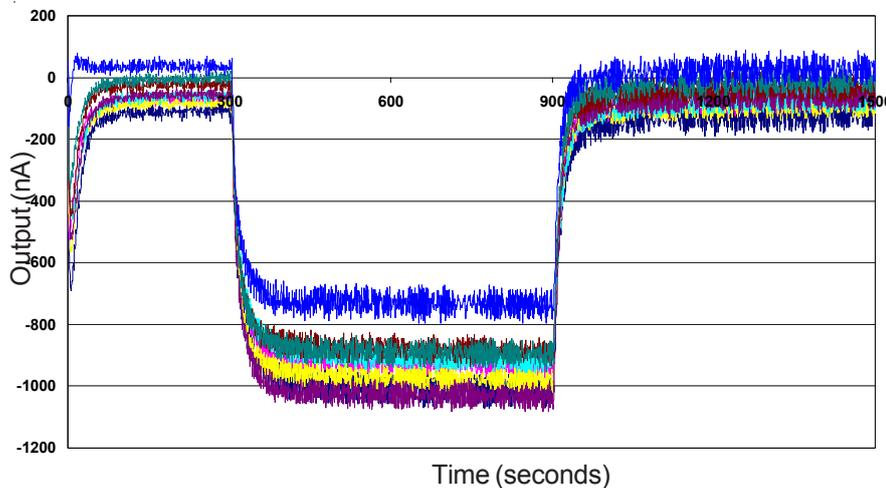
When designed with a 22 ohm load resistor, the NO2-B1 shows excellent resolution, even at the ppb level: ideal for outdoor air environmental testing.
