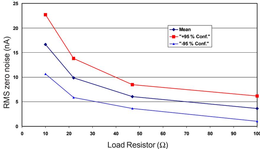
Figure 3 shows the effect of load resistor value on the RMS zero noise for the NO2-B1 sensor.
