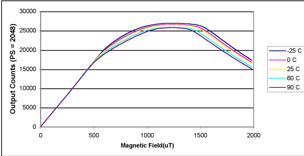
Figure 3-1: Temperature Characteristics
