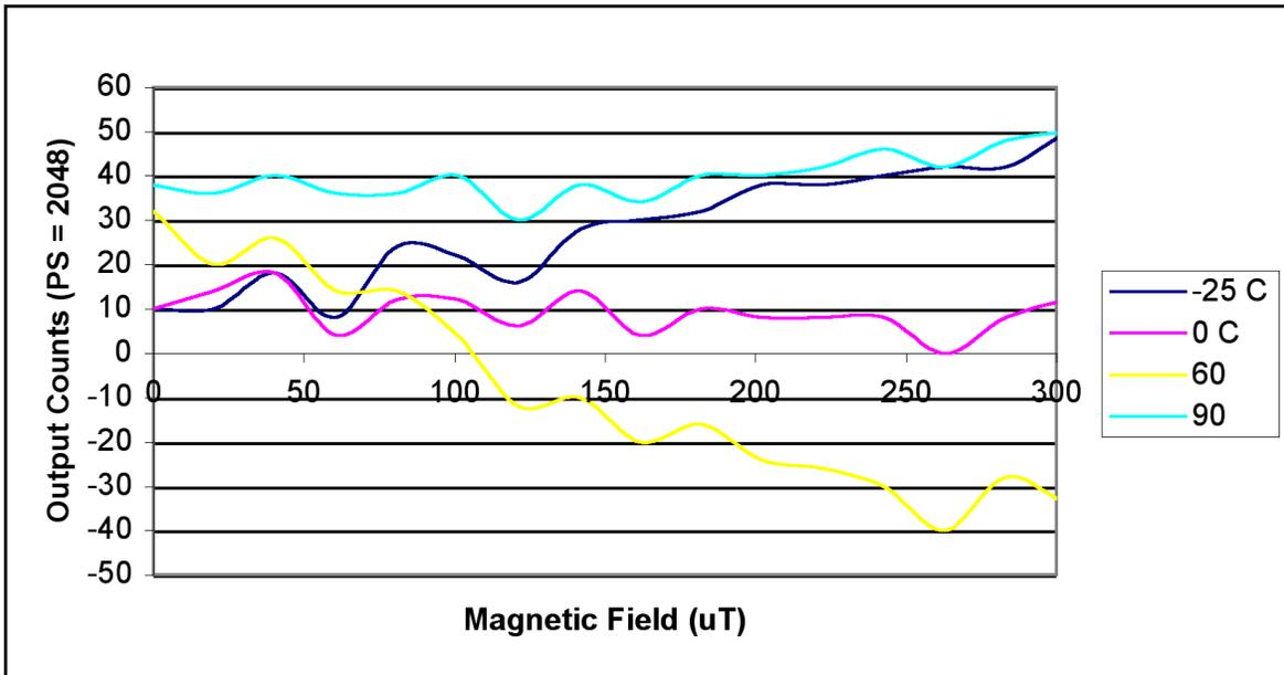
Figure 3-3: Linearity vs. Temperature, Normalized to Room Temperature
