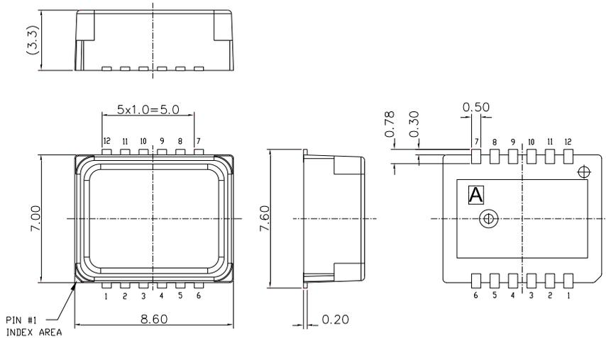
Figure 3. Housing dimensions
