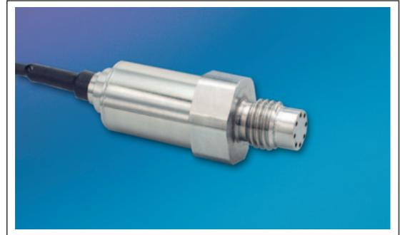
The ET-5DC-312 series is designed to measure barometric pressure from ground level to 30,000 feet. The ET-5DC-312, is designed with Kulite's latest dielectrically isolated Patented sensing element, coupled with a microprocessor providing a digital compensation, analog output signal. The unit is ideally suited for applications where accuracy requirement is a prime importance.
